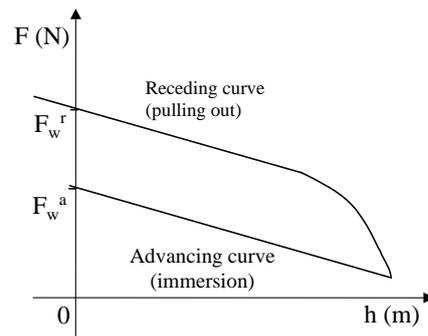
Figure 2. Forces recorded by the tensiometer as a function of immersion depth ( $h$ )
